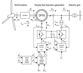
Fig.1. Wind turbine control system with DFIG
