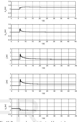
Fig. 10. Response characteristic at sudden wind speed changes;  $v_{w1} = 0.0[m/s], v_{w2} = 6.0[m/s], p_{ra}^* = 0.1[pu], K_{pr} = 30.0, K_{ir} = 0.015$
