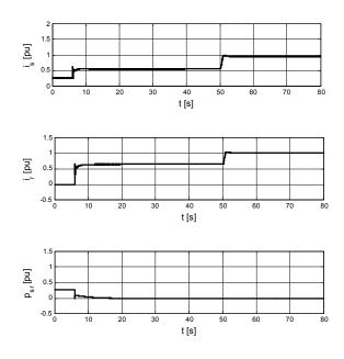
Fig.8. Time responses with the rotor active power regulation;  $K_{pr} = 100.0$ ,  $K_{ir} = 0.05$ ,  $p_{ra}^* = 0.0[pu]$ .
