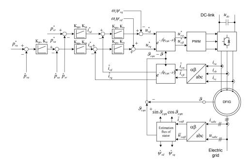
Fig. 4. Active and reactive power vector control system of DFIG with rotor power feedback control
